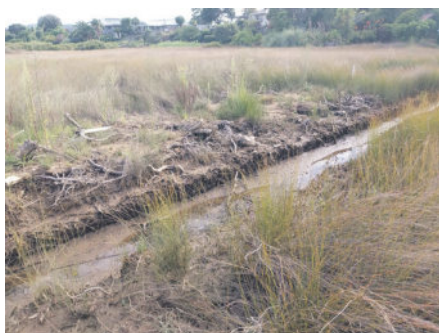
At the inlet, fine sediment mixes with sand and organic material, forming a dense substrate that does not easily re-separate once settled.
