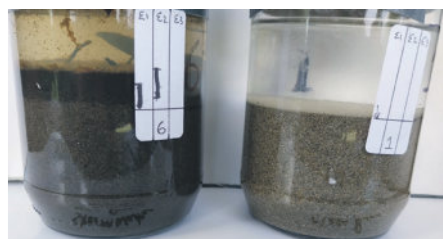
Jar tests from different parts of the system: clean sand, fine sediment, and the mixed material that forms when the two combine.
