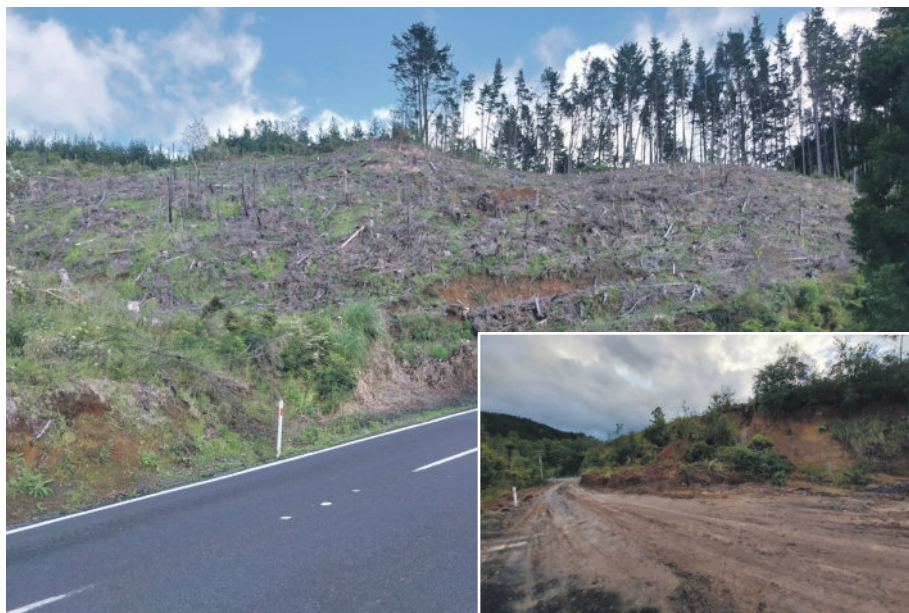
Exposed ground during disturbance phases increases the mobilisation of fine sediment during rainfall events.
