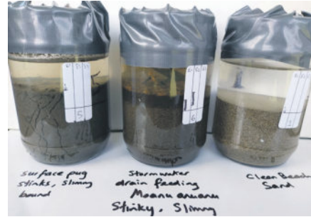
Jar separation tests showing sludge.
